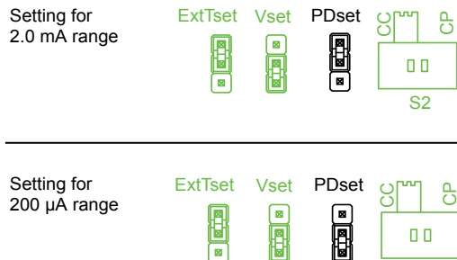
Figure 8. Select the photodiode range with the PDset jumper.
